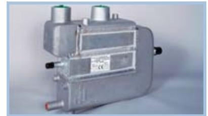
Designed specifically for air dryer OEM's, the all-aluminum brazed PCR combines a regenerative economizer with a refrigerant cooling section and a built-in moisture separator to provide the most compact, efficient 3-in-1 heat exchanger available. Capacities from 76 to 600 SCFM @ 100 psi with exiting RH below 25%.
