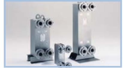
The Sigmawig all-welded plate heat exchanger has operating temperatures as high as 750° F and as low as -320° F, and operating pressures as high as 360 PSI. The unique concept of this rugged heat exchanger makes it a viable solution for many heat transfer needs previously thought only suitable for shell & tube designs.
